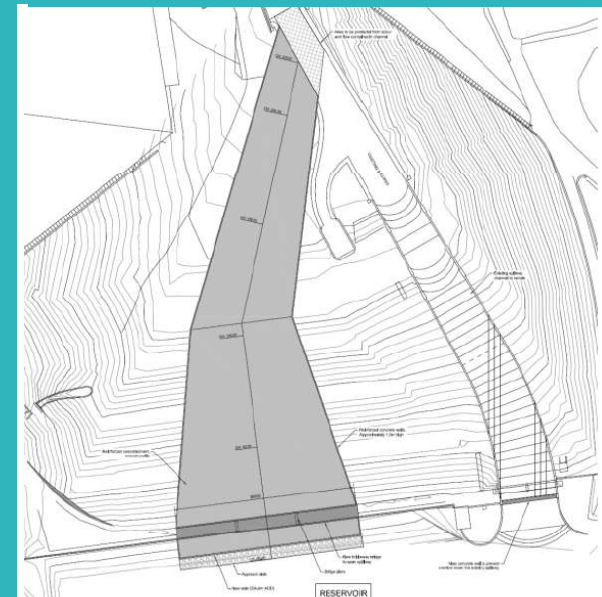
Over embankment spillway
